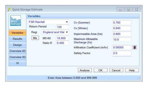
Figure A1 Microdrainage Source Control Quick Storage Estimate Input
